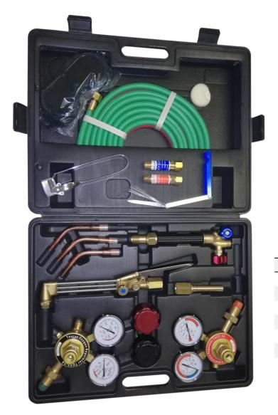
The TAURUS combination kit is a starting kit for general brazing, welding and cutting with oxygen and acetylene gas. It can be extended to suit personal and job requirements. The equipment is presented in a secure, robust toolbox. The inlet fittings on the regulators are G 5/8" - B-rh on the oxygen side and B-lh on the acetylene side. The fittings are compatible with industrial size gas cylinders in South Africa.
