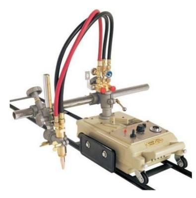
The straight line cutter CG1-30 is a light, portable machine running on rails which can be extended to suit the cutting length. It uses oxygen-acetylene or oxygen-LPG. The traveling speed is adjustable enabling cutting through materials up to 100mm thick. Cutting nozzles ANME/ANM and PNME/PNM used on the universal cutting torch, can both be fitted to the machine.
