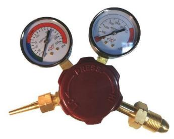
The primary function of a gas regulator is to reduce high-pressure gas in a cylinder or process line to a lower, more usable level. A regulator is not a flow control device. It is used to control delivery pressure only. It has two gauges, one to measure the inlet pressure and the other to measure the outlet delivery pressure.
