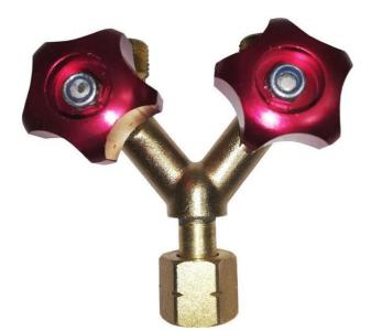
The TAURUS Y-PIECE with valve fittings has a single-line inlet and dual-line outlet connectors allowing two hoses running from one gas regulator source. The dual outlet connection is fitted with two valves allowing independent control of each line.
