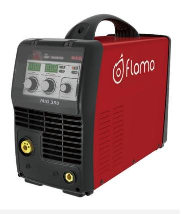
The Flama MIG 350-3 is a compact 350A, MIG welding machine. Its inverter technology design is ideally suited for demanding industrial applications. The sturdy internal wire feeder can accommodate wire spools up to 20kg in weight. This robust machine has phase-loss protection, a high duty cycle, and a soft arc. It therefore, ensures easy welding and produces high quality welds. This machine is ideally suited for the professional welder.
