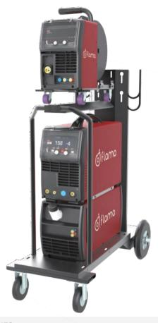
The Flama MIG 500F synergic is a 500A multi-purpose welding machine. Its inverter technology design is ideally suited for demanding industrial applications. The sturdy internal wire feeder can accommodate wire spools up to 20kg in weight. This robust machine has phase-loss protection, a high duty cycle, and a soft arc which ensures easy welding and produces high quality welds. This machine is ideally suited for the professional welder.
