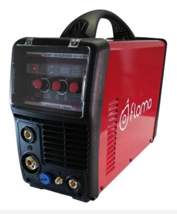
The Flama MULTIMIG 180EX is a 180A multi-process MIG inverter machine. The machine's inverter technology design is ideally suited for demanding industrial applications. It is a compact, versatile welding machine with capacity for MIG, lift TIG and MMA welding processes. The feeder supports up to 5kg wire spools making the machine conveniently portable for field operations. The Flama MULTIMIG 180EX delivers clean, high-quality welds to the satisfaction of professional welders.
